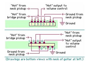
If you want to be more flexible, you can use the Fender 4-way Tele switch as shown in the circuit below. This will give you both sounds when choose the two pickups together - wired in parallel (standard wiring) and the new wired in series sound.
