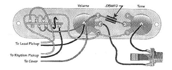
You can also use an additional switch for this option together with the standard 3-way Tele switch. Have a look at the circuit below. The 3-way switch will stay the same and position #3 (bridge pickup alone) + activating the switch will give you both pickups wired in series. Naturally you can also use a push/pull pot for this.
