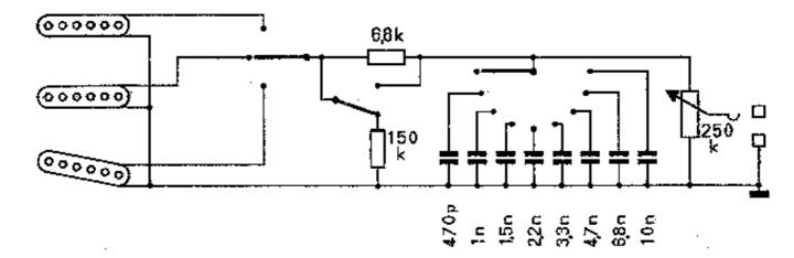
Feel free to use this basics and go wild ...... you can add some more switches to choose between different types of caps and resistors, rotary switches for more than 8 cap values, add an additional pot after this complete structure to have even more control about each individual cap that is dialed in (see circuit above) ......
